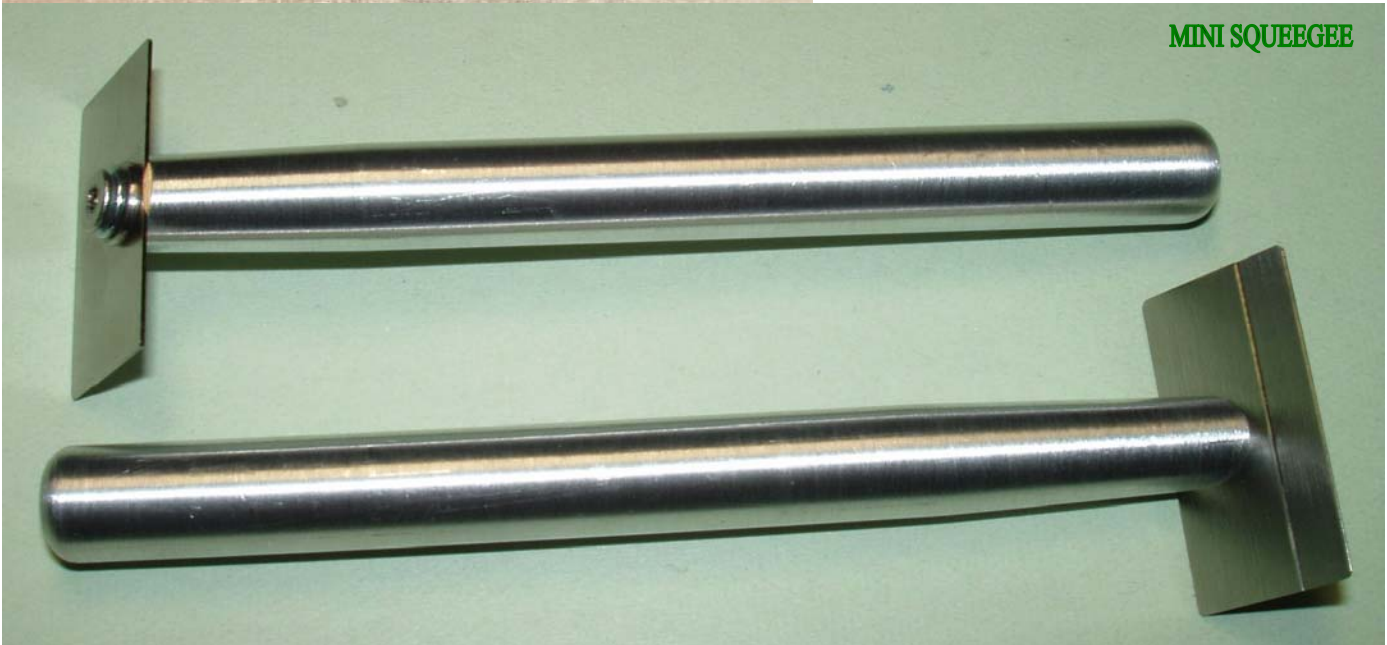
Stapula for BGA paste/flux application. 19cm length
